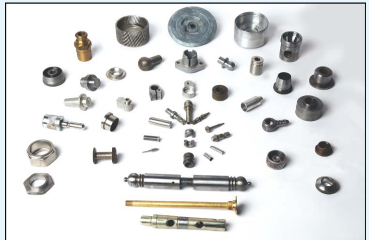
Components Manufactured on SUMANGAL automats
